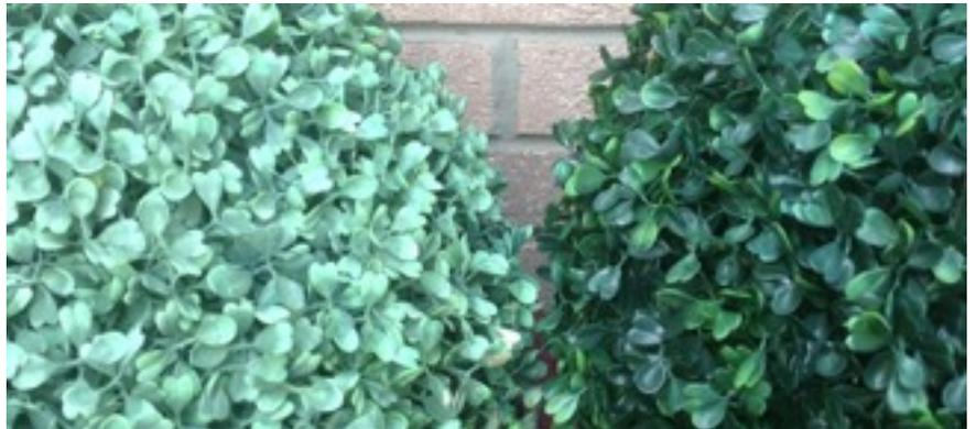
Comparison of UV inhibited and non-UV inhibited foliage with similar environmental exposure
